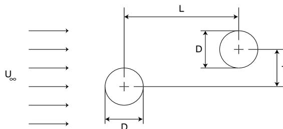
Fig. 1. Configuration of cylinder pair.
