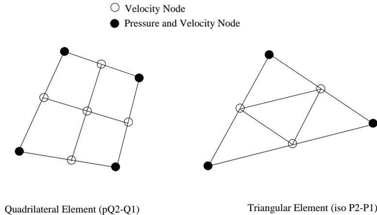
Fig. 3. Quadrilateral and triangular mixed elements.
