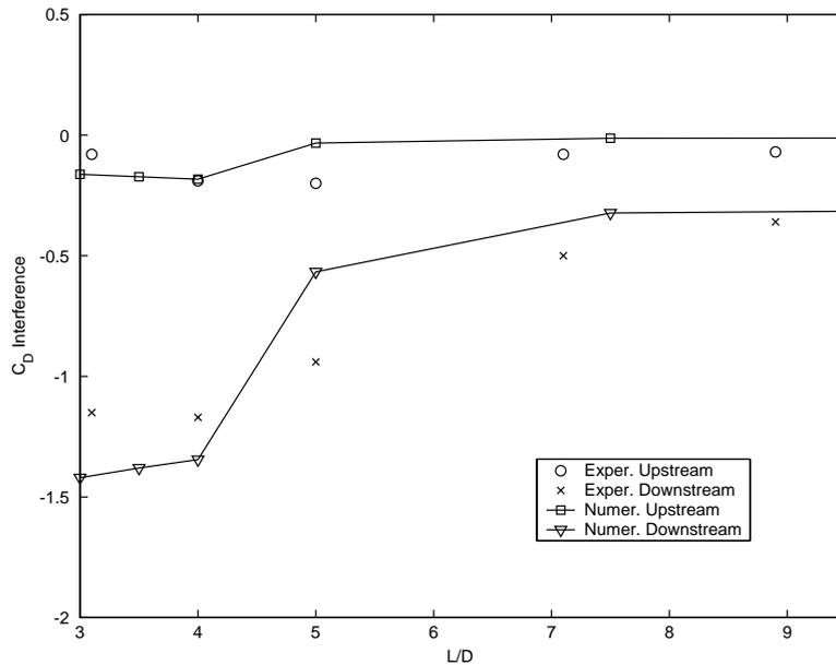
Fig. 4. Interference drag for tandem cylinder pairs at  $Re = 80$ . Comparison with experimental results of Tanida et al., 1973.
