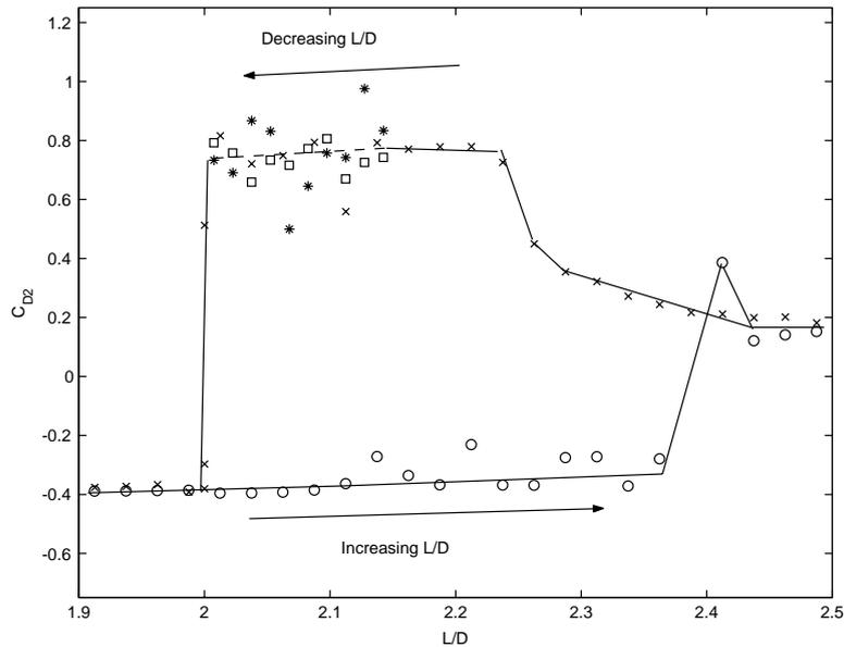
Fig. 9. Hysteresis of downstream drag coefficient,  $Re = 1000$ .Table 1
