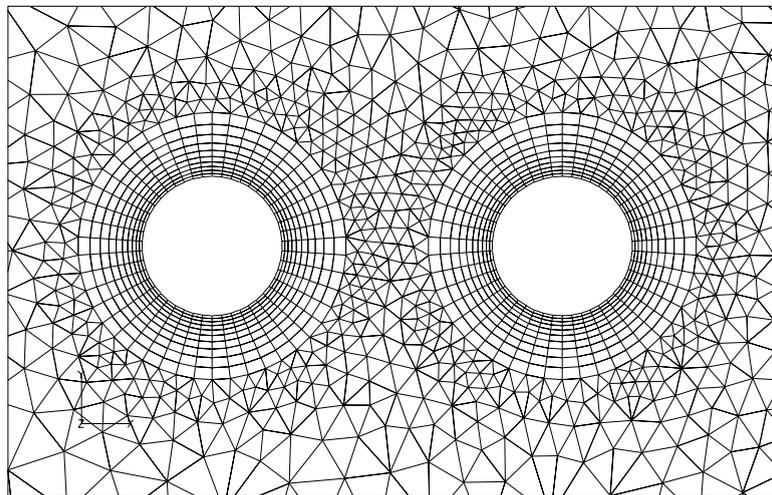
Fig. 2. Closeup of hybrid mesh for a cylinder pair.
