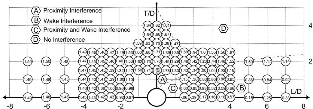
Fig. 12. Mean drag coefficients for  $Re = 1000$  staggered arrangements with boundaries of interference regimes.
